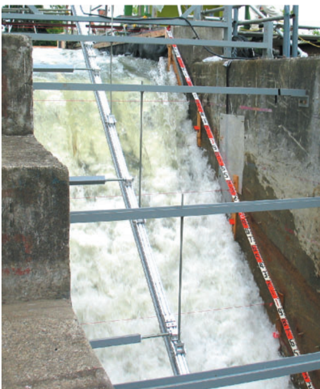
Figure 19. Stream regime on downstream side at overflow level 2 at q = 0.348 \text{ m}^3/\text{s/m} , h_0 = 0.323 \text{ m}
