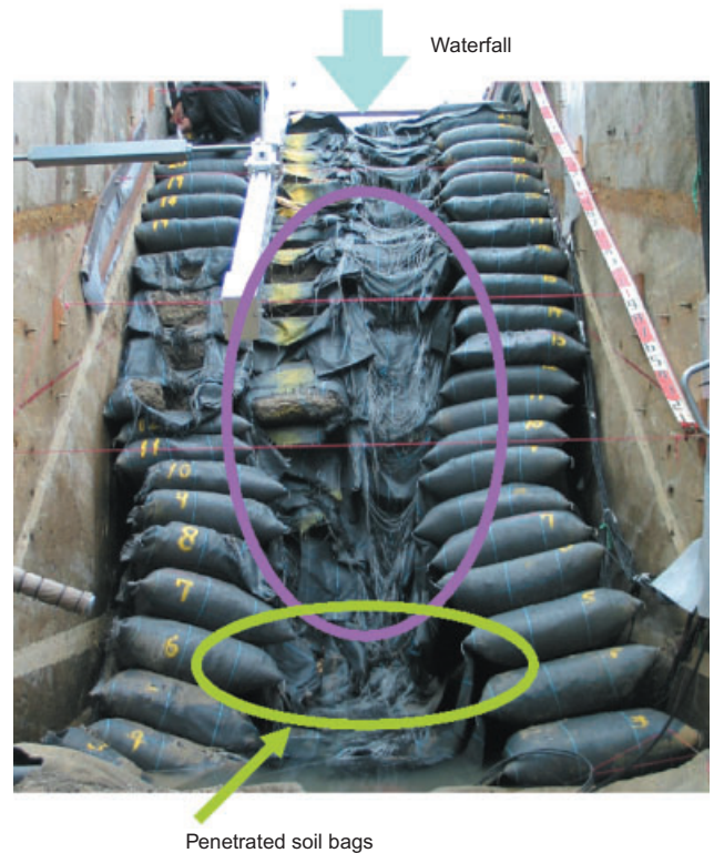
Figure 23. Erosion trace like the formation of a waterfall basin after final overtopping
