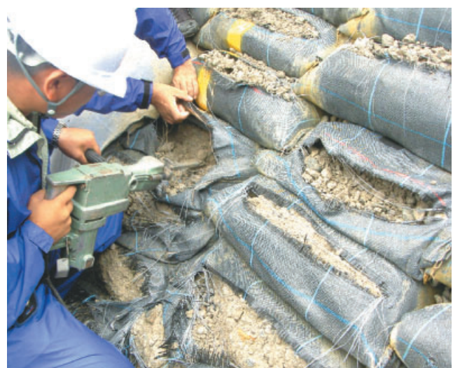
Figure 21. Artificial physical damage: cutting surface of geotextile soil bag, and loosening backfill material
