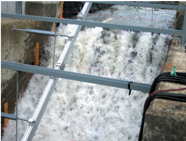
Figure 18. Stream regime on downstream side at overflow level 1 at q = 0.087 \text{ m}^3/\text{s/m} , h_0 = 0.190 \text{ m}
